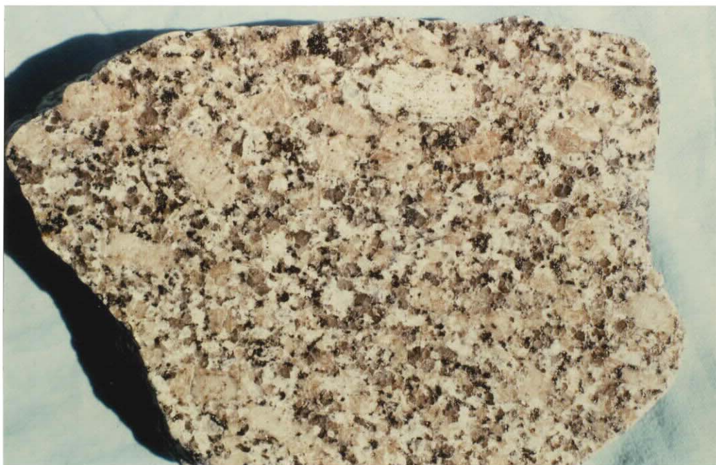
PLATE 2. Polished slab of Boree Rocks porphyritic adamellite. Slab is 15 cm across.
