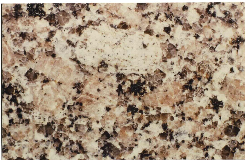
PLATE 3. Close up of porphyritic adamellite. Pink phenocrysts of orthoclase are enclosed by matrix of plagioclase, quartz and biotite. White spotted xenolith is 2.5 cm long. Slide No. 35147
