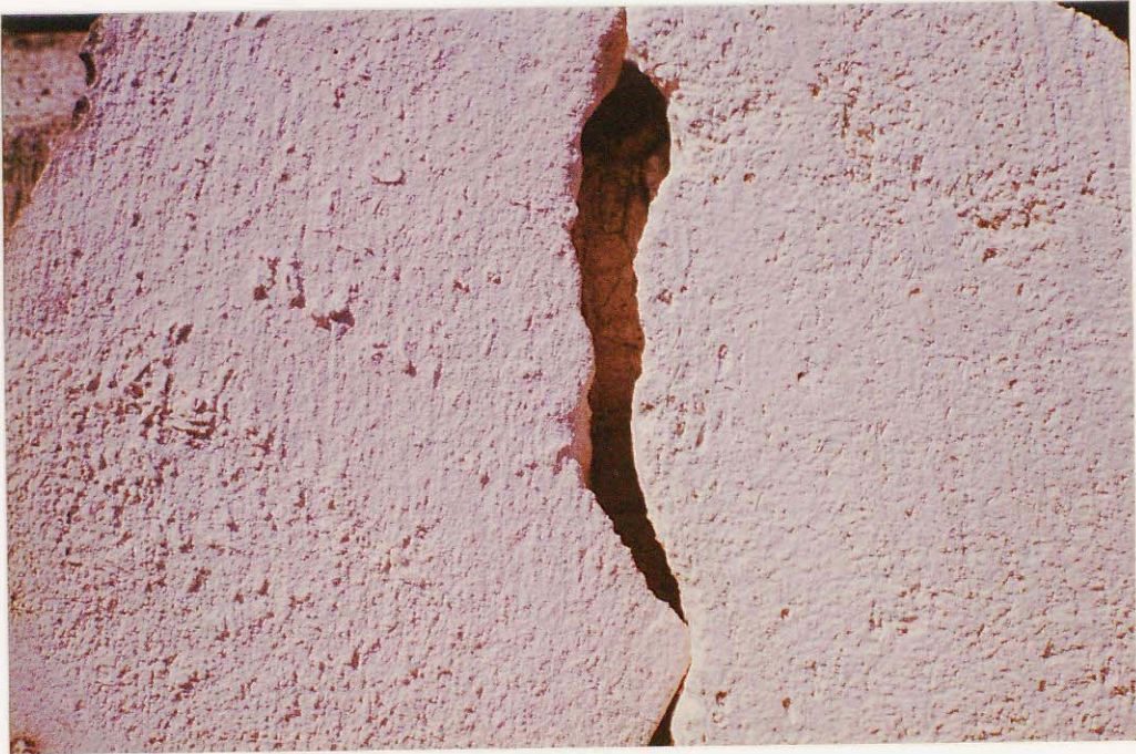
PLATE 10. Gambier Limestone from Honeysuckle Flat (left) and Marte. Note slight grey-brown tinge to Honeysuckle Flat limestone.
