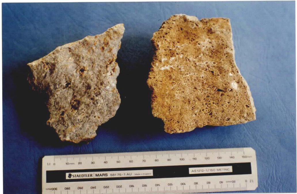
PLATE 9. Vuggy calc-dolomite near base of upper member, Wilkawillina Limestone. November 1983. Slide No. 24354.
