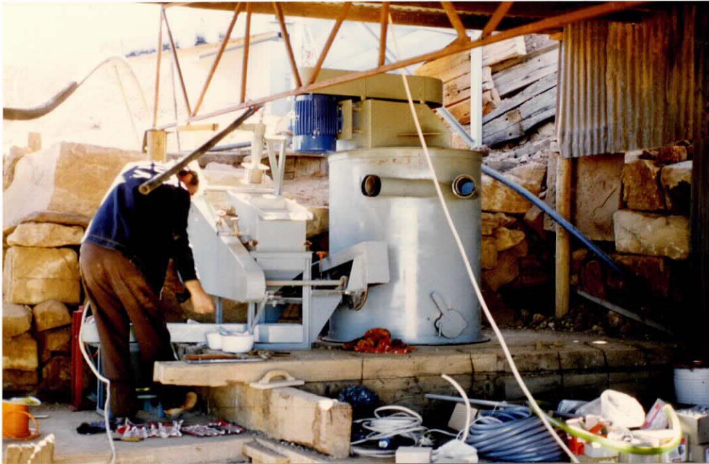
Plate 3. Agitator unit fed with material from the screens behind. (photo No. 34491)
