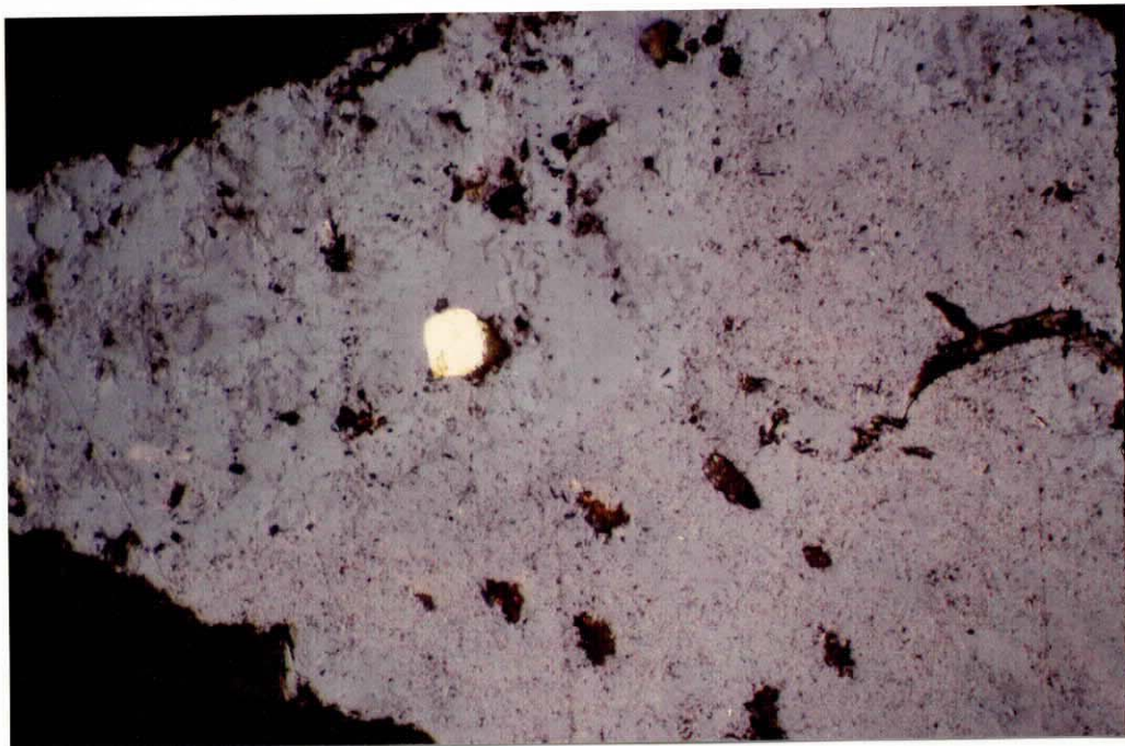
Plate 7. 10 \mu m gold grain in goethite. Field length 0.5mm Polished Sect. 33679 Sample A 2628/84. (photo No.34496)
