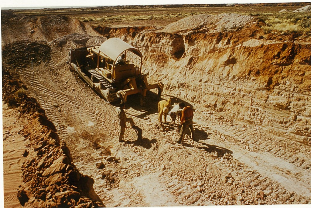
PLATE 6 - Bulldozing, Andamooka 1976, 'opal level' at 3.5 m below surface being checked by miners adjacent to Subsidised Shaft 5. (slide 13755)
