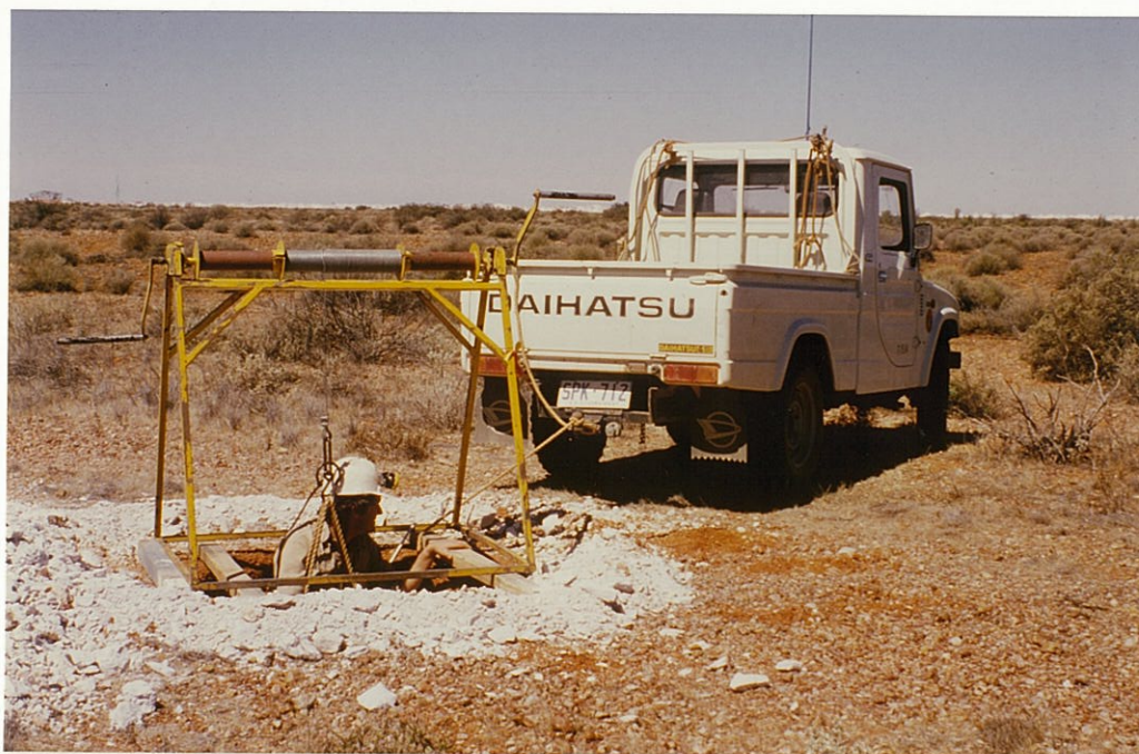
PLATE 22 Mapping Subsidised Shaft 98 Coober Pedy, October 1981. Lightweight hand windlass used to lower geologist down Calweld shaft. (slide 24732)
