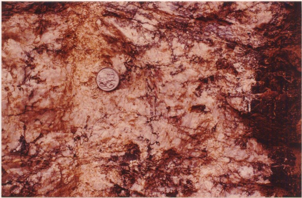
PLATE 5. Beltana No. 2 Lode - white, coarse-grained barite on west side of face at base of northern access ramp. Black goethite as staining along irregular fractures and in band on right. October 1983. Slide No. 24459.
