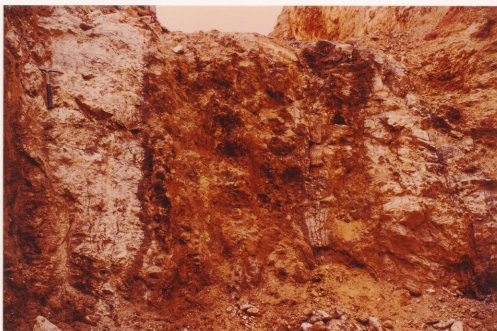
PLATE 4. Beltana No. 2 Lode - barite lode 3.5 m wide on face at base of northern access ramp. Dark botryoidal goethite forms distinct bands parallel to lode margin which dips steeply easterly. Central portion consists of extensively ferruginised barite with yellow goethite. October 1983. Slide No. 24458
