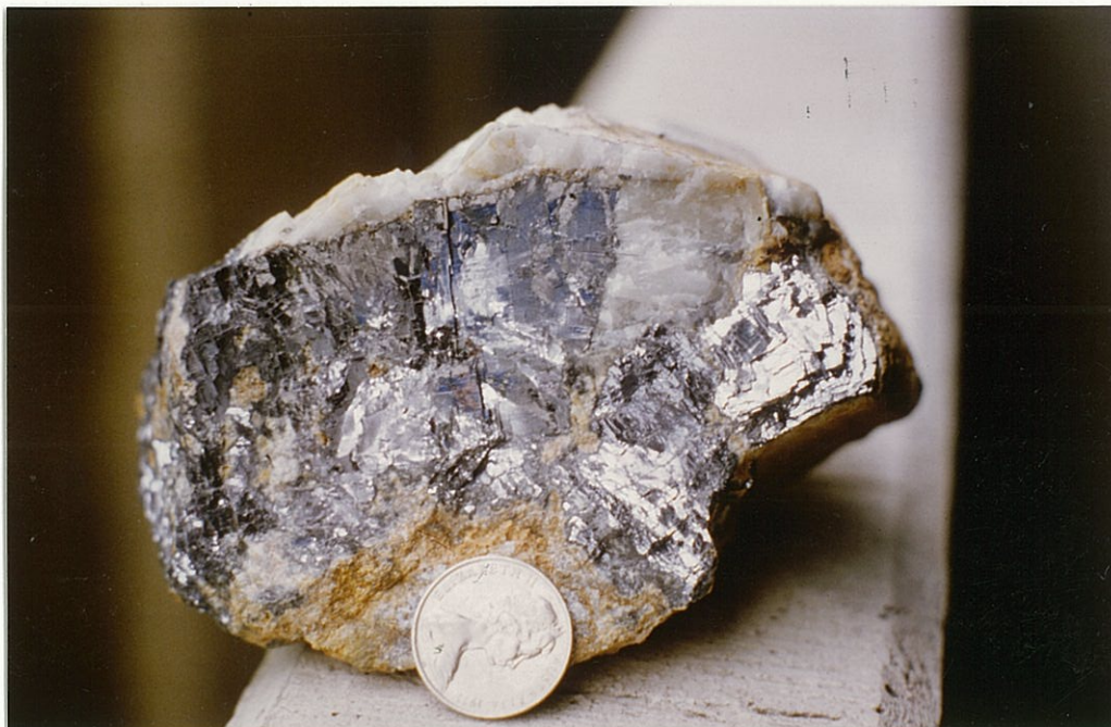
PLATE 3 Typical massive galena ore with barite from Wheal Gawler. Trans. No. T24192
