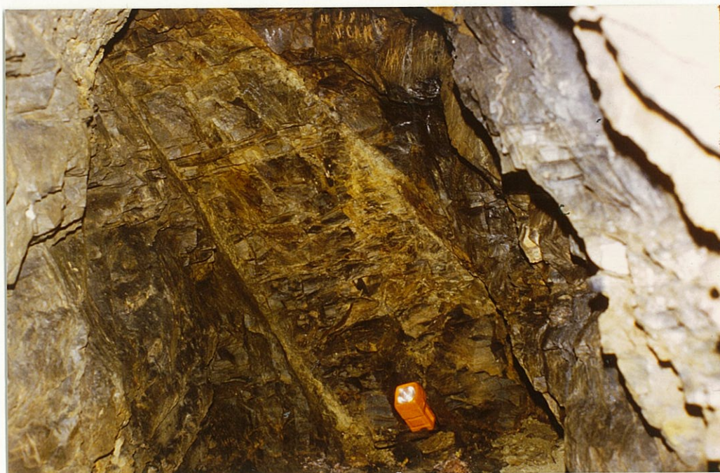
PLATE 5. Steep northerly dipping fracture zone in calcareous siltstone at the end of the Deep Cross Cut, Wheal Gawler. Trans. No. T24194
