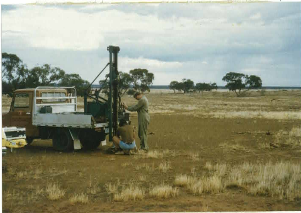
PLATE 2. Craigie Plains Gypsum Deposit No. 2. Daihatsu tray-top mounted auger drill at work. (April, 1981) (Photo No. 33320).
