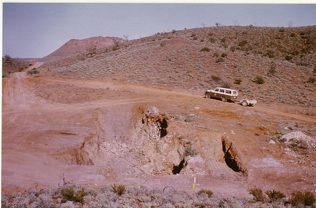
PLATE 2. Nilpena 1D Lode. View southwest. Lyfords Cut is behind and left of survey peg, with deep footwall cut further left and small hanging wall cut to the right. Prominent strike ridge in background formed by ABC Range Quartzite. (June 1979). SLIDE NO. 23143.
