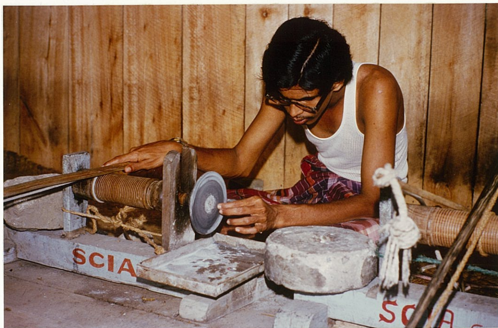
PLATE 5. Dressing and shaping rough gemstones using an abrasive wheel rotated by a bow string. Trans. 22998
