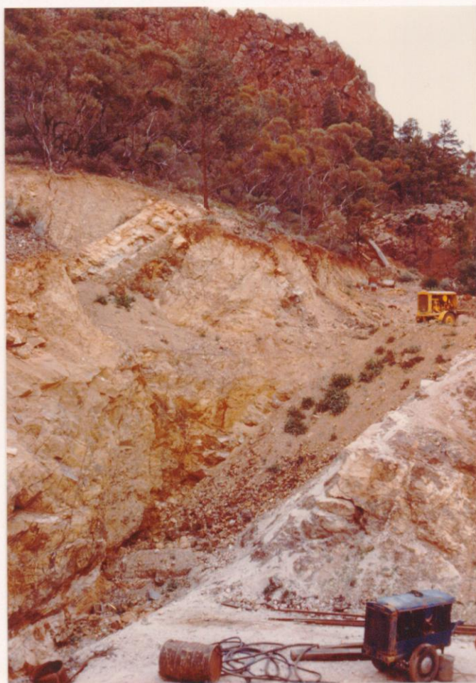
PLATE 1. McRae Deposits - No. 1 Lode. View eastwards from main workings, 670 m bench in foreground. Easternmost pit in mid distance, massive, boldly outcropping, Wilyerpa Formation quartzite on skyline. Fault displaces barite lode, from yellow compressor on 680 m bench, 20 m to the left. (June, 1979). Neg. No. 32485
