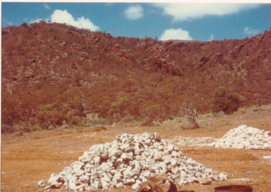
PLATE 4. McRae Deposits - No. 2 Lode View eastwards from campsite to No. 2 Lode on slopes of Loves Mine Range. Barite stockpiles in foreground; oil drilling grade on left industrial grade on right. (March 1979) Neg. No. 32488
