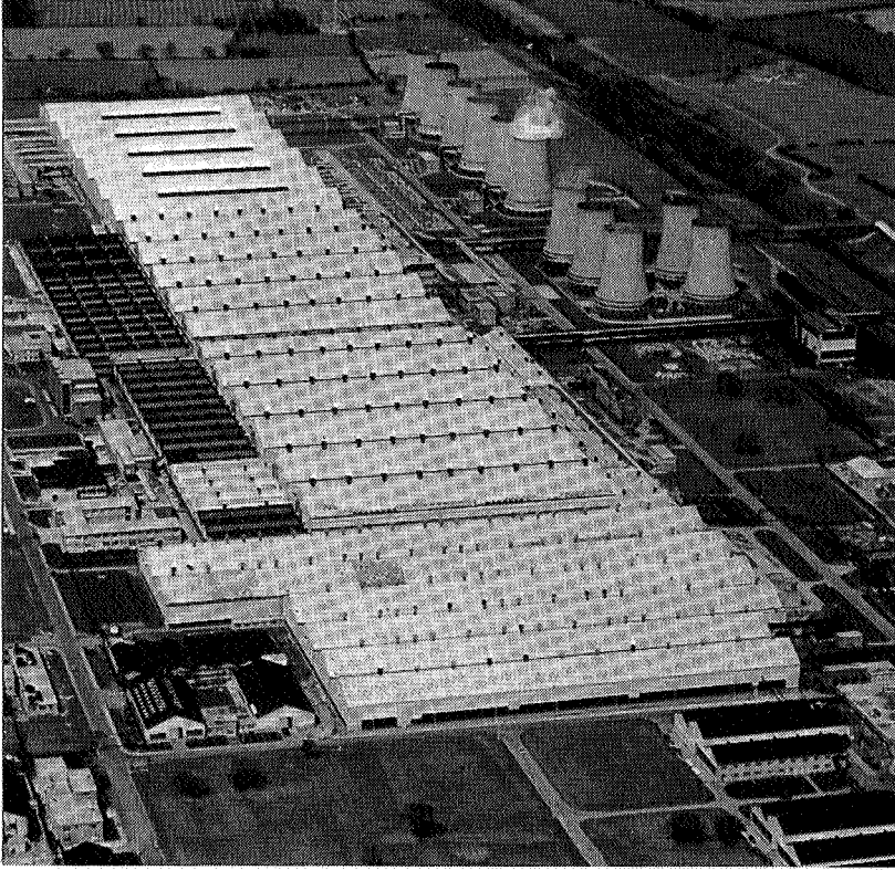
BNFL - Capenhurst gaseous diffusion plant (the adjacent centrifuge enrichment plant occupying less than one quarter of the area of diffusion plant is out of picture, left centre)
