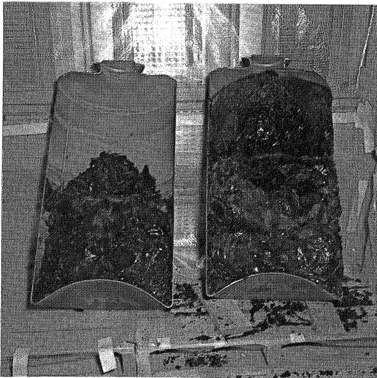
Canisters sectioned to illustrate storage simulation of vitrified fission products (AVM)
