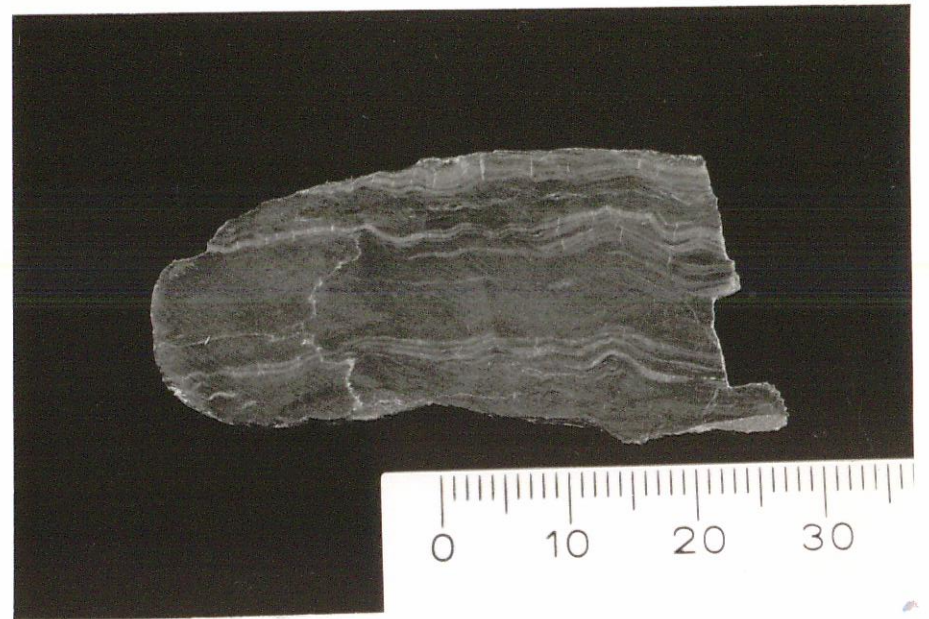
Fig. 3 (a) Outcrop in Mindrow Creek of mylonitized gneiss on the right grading into slaty mylonite on the left. (b), (c), (d) Mylonitic gneiss specimen MY-1, mylonite specimen MY-4 and slaty mylonite specimen MY-6 collected from the right, the centre and the left, respectively, of the outcrop shown in (a). The scales are in mm.
