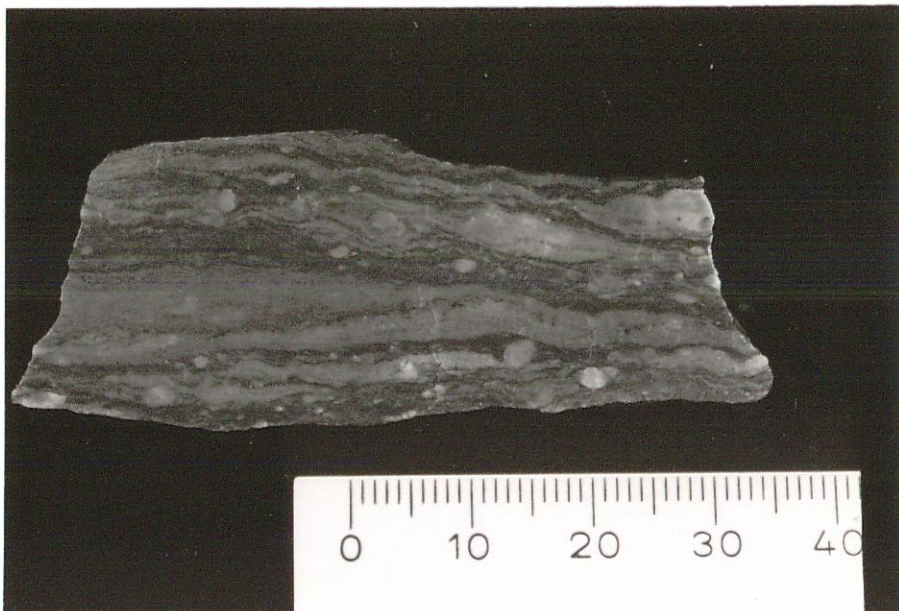
Fig. 3 (a) Outcrop in Mindrow Creek of mylonitized gneiss on the right grading into slaty mylonite on the left. (b), (c), (d) Mylonitic gneiss specimen MY-1, mylonite specimen MY-4 and slaty mylonite specimen MY-6 collected from the right, the centre and the left, respectively, of the outcrop shown in (a). The scales are in mm.
