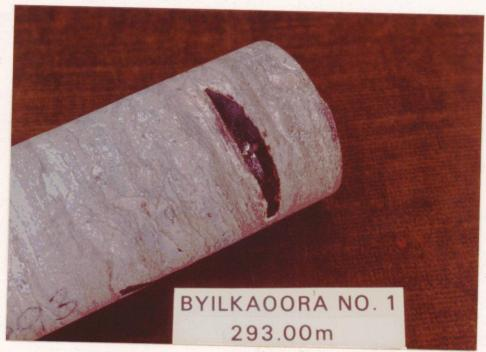
PLATE 4 Core segment showing oil biodegraded to a bitumen within a vug in dolomite rock. (Core is 48 mm diameter, arrow point downwards).
