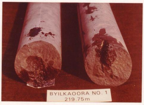
PLATE 2 NQ drillcore from 219.75 m depth, showing oil bleeding from calcite veins and a calcite and pyrite-lined vug. (Transparency No. 14752; Neg. No. 30877).
