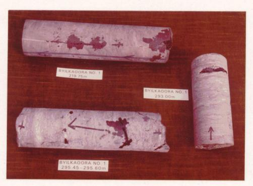
PLATE 3 Selection of core segments, showing "bleeding" oil in dolomite. (Core is 48 mm diameter, arrow points downwards).
