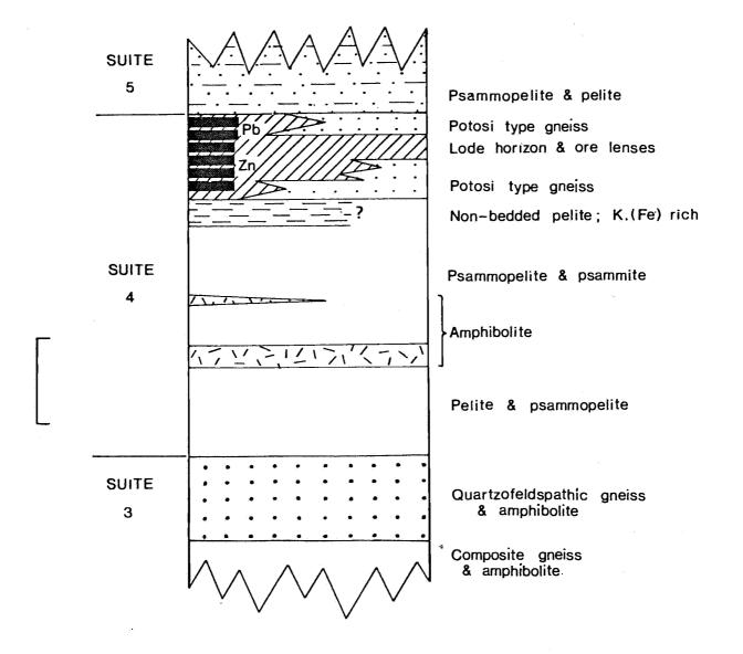
Fig. 7. Composite stratigraphic section of the Broken Hill mine sequence in the mines area. Bar scale is approximately 100 m. From W.P. Laing in unpublished report GS1979/062, Geological Survey of New South Wales.
