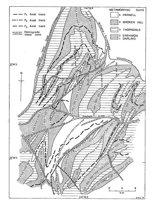
Fig. 6. General geology of the Broken Hill subdomain in the Willyama orogenic domain, showing inferred axial traces of superposed folds of three generations. Redrawn from map prepared by N. Archibald as part of the Broken Hill Lode Horizon research programme at the Department of Earth Sciences, Monash University. Unpublished geological information from the N.S.W. Geological Survey is included.
