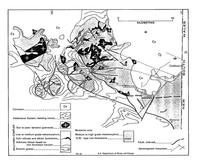
Fig. 5. Regional geology of the Olary subdomain. A complex system of curved, branching shears determines the relative distribution of Willyama Complex and Adalaidean rocks. As a consequence, individual fault-blocks or inliers of Willyama Complex are bounded to the west by shears and to the east by unconformably overlying Adelaidean rocks. This pattern is maintained throughout the Willyama Domain.
