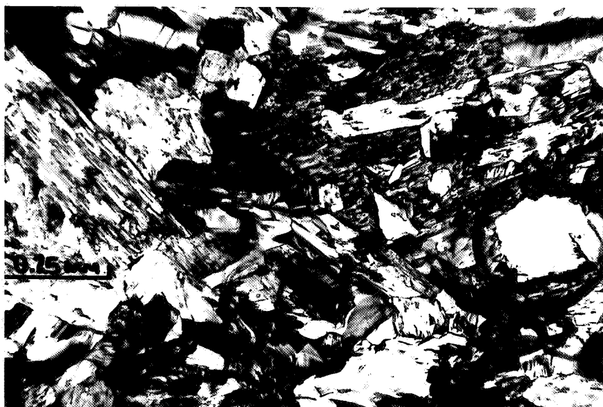
Plate 8. Elongate secondary gypsum crystals in vein. Wilkinson No. 1, 326.7 m (From acetate peel).
