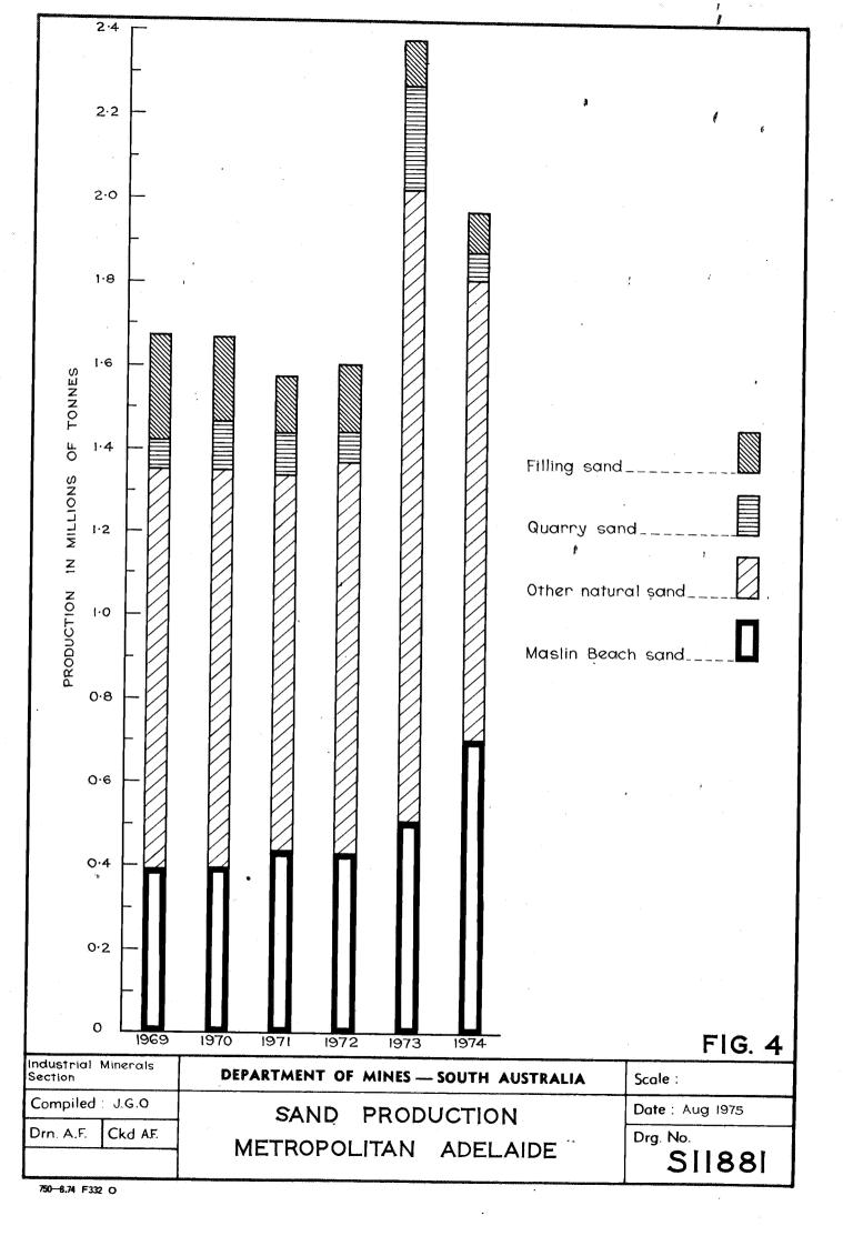
At Maslin Beach, both washed and unwashed sand is produced for use as concrete fine aggregate, mortar and plastering. At one stage, foundry sand was supplied to Chrysler Aust. Ltd. from Christies Sand Pit. However, the size grading of this material was too variable. A classification plant is required to produce consistent graded sands for special uses.
