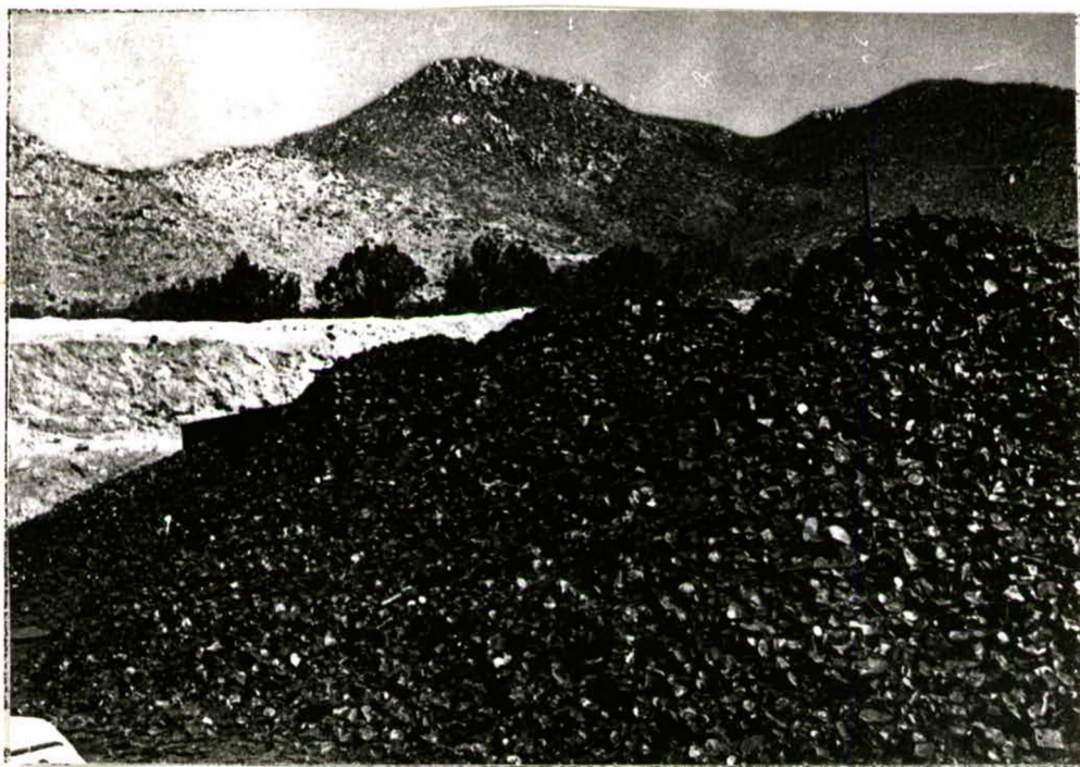
FIGURE 23. - Stockpile of Partially Oxidized, Burned, and Shredded Cans at Mineral Park Precipitation Plant, Duval Corp. Brown color is typical of the oxidized detinned and shredded cans.
