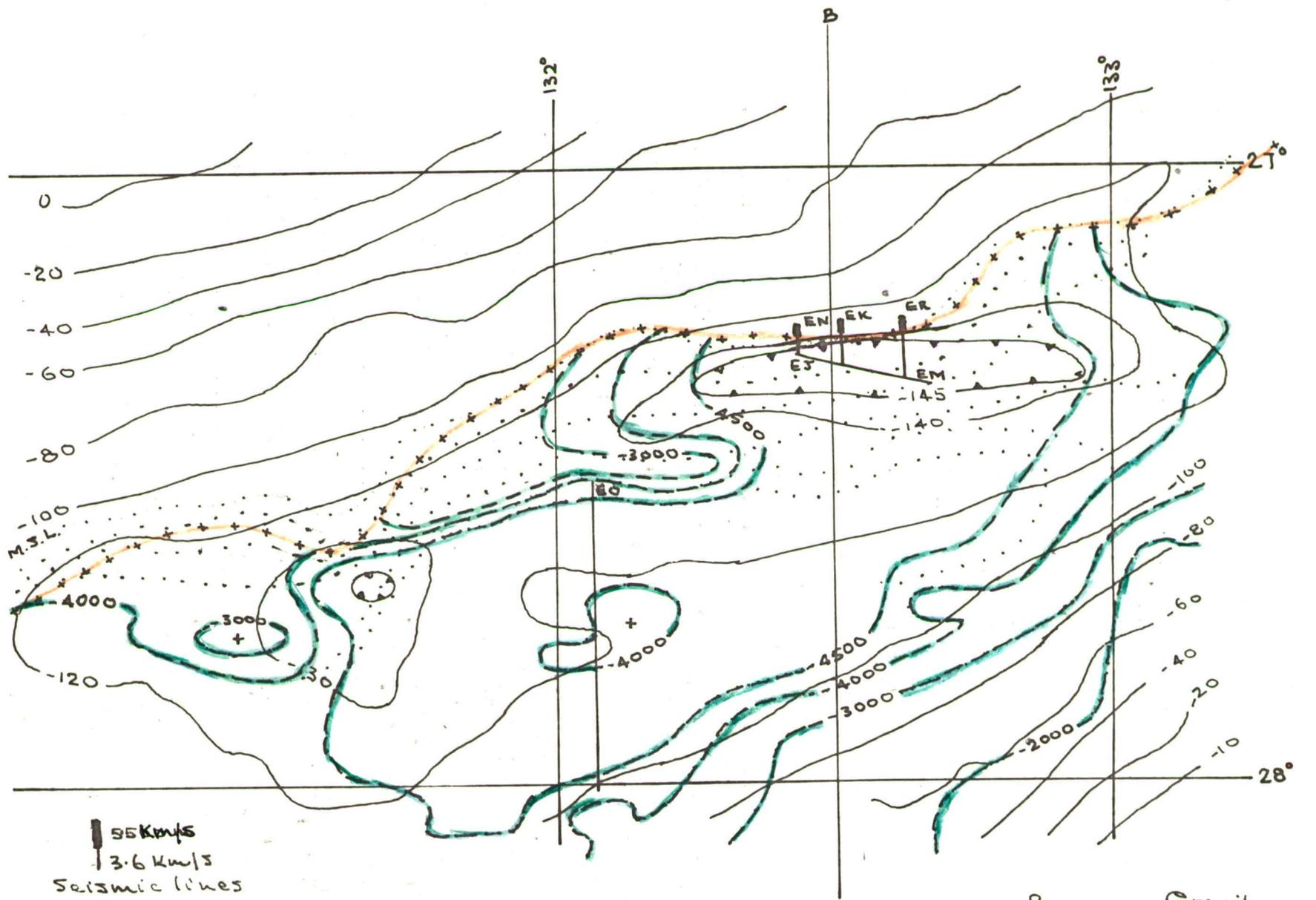
Fig.1 EASTERN OFFICER BASIN - Contours of Bouguer Gravity and Depth to Magnetic Basement
