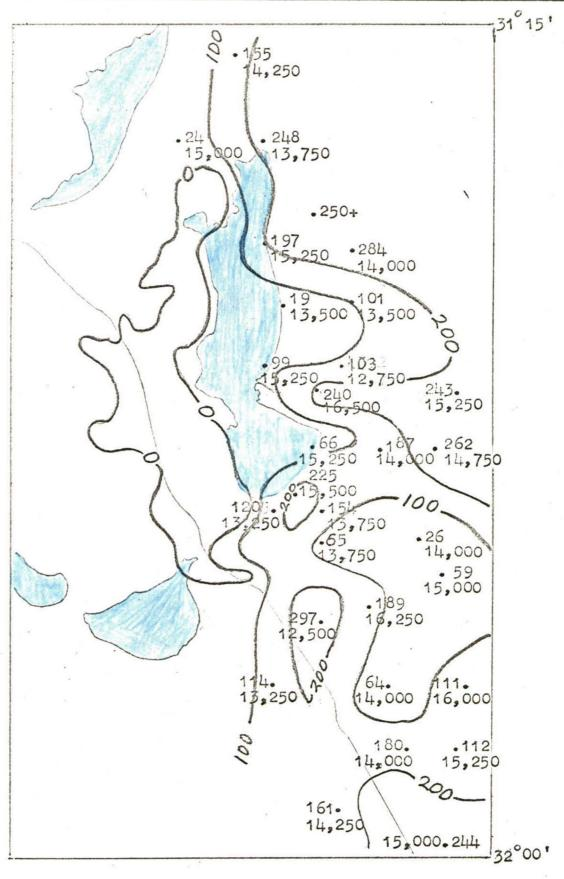
Seismic spread position showing depth & velocity of high speed refractor (Depth in feet, velocity in feet/second) 14,000
