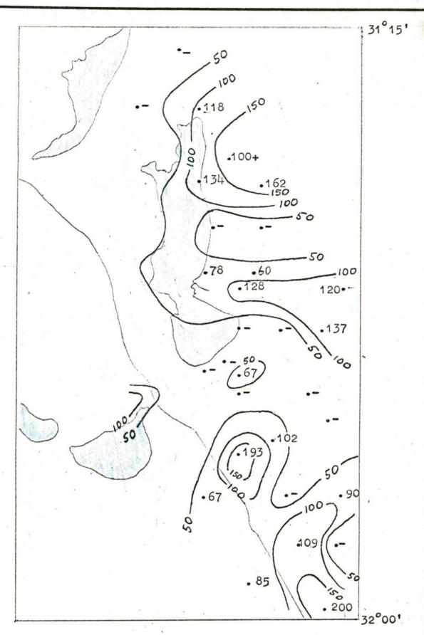
Seismic spread position showing thickness of intermediate velocity (9000-12500 fps.) refractor. Thickness in feet
