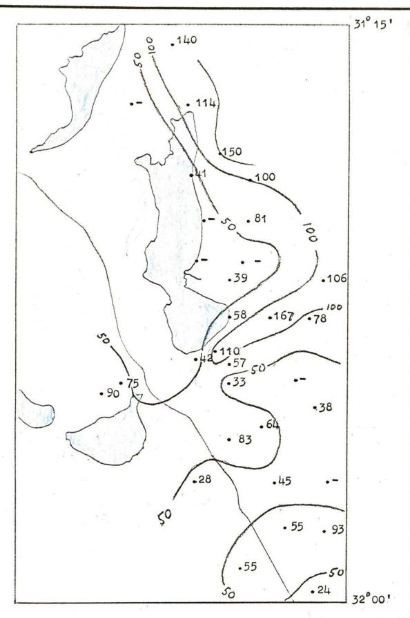
Seismic spread position showing thickness of low velocity (5,000-9,000 fps.) refractor. Thickness in feet
