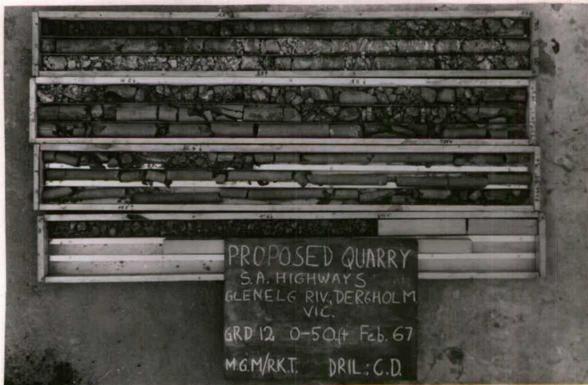
Fig. 2 Core from diamond drillhole GRD 12 showing all degrees of weathering - clay at top and bottom, fresh basalt in the middle. Scale 1 in. = 1ft.
