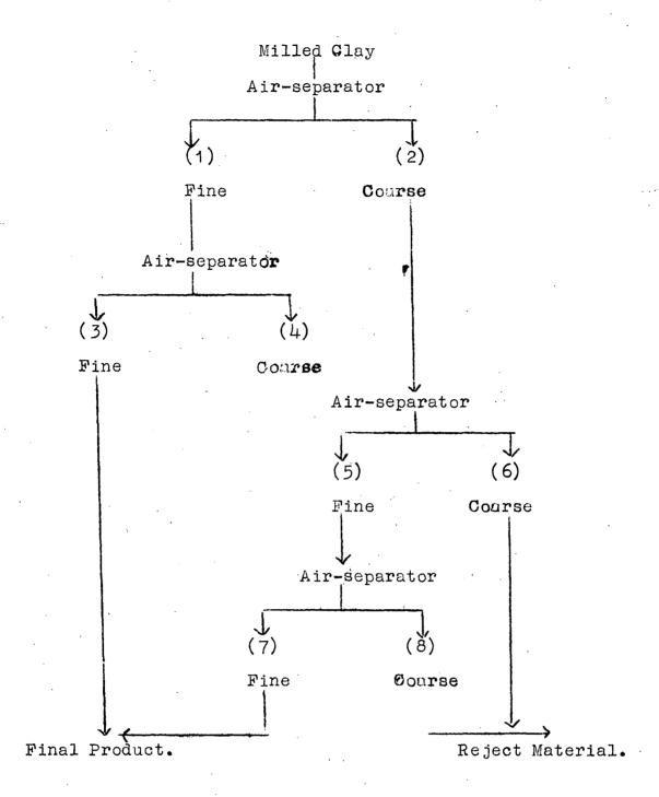
The operation of flowsheet 1 resulted in a final product (Nos 377) representing 62.5 per cent by weight of the feed.
