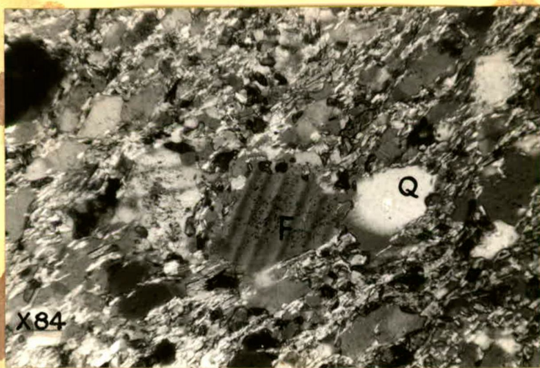
FIG.1 Greywacke showing irregular grains of quartz and feldspar surrounded by muscovite and biotite. Note lineation.
