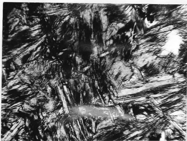
(b) Decussate aggregates of fibrous crocidolite in tough segregations of crocidolite marble from Section 30, Hd. Bright (Hallelujah Hills). Interstitial minerals are albite and dolomite.
