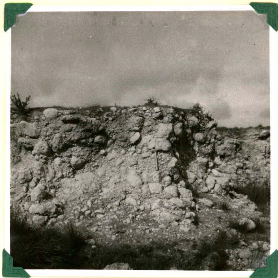
Fig. 13. Nodular travertine typical for the road metal quarries in the area (Hd. Wallaroo)
