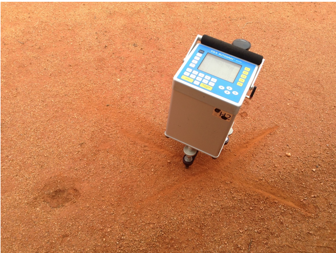
Figure 13. The GPS vehicle surveys the points and marks the ground over which the gravity is recorded. (Photo 414130)
