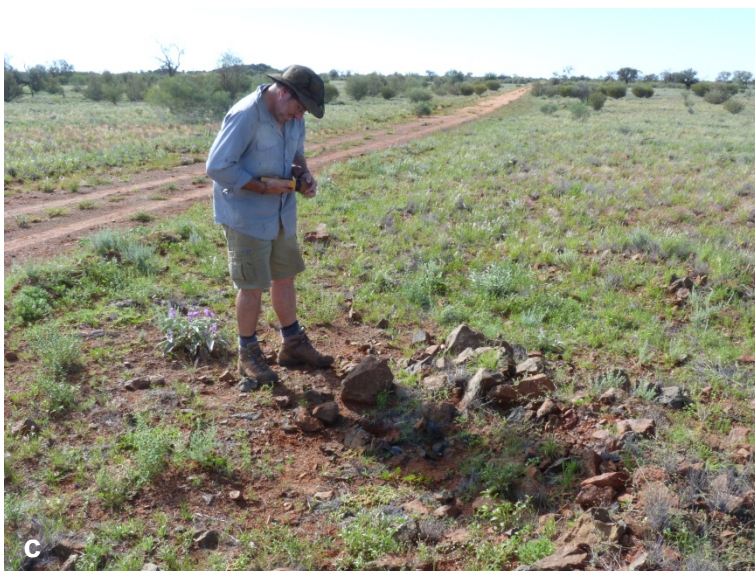
Figure 3. a) Using the Ultramag Geophysics GSM-19 magnetometer along a station track on traverse 4. b) Marking out the traverse and recording data in a field tablet PC. c) Using a KT-9 magnetic susceptibility meter on a sample of gabbro from traverse 3. (Photos 414101–414103)
