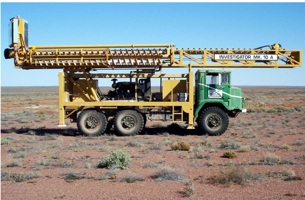
Plate 2. Coober Pedy Miners Association MK 10A auger drilling rig. (Photo No. 404950)
