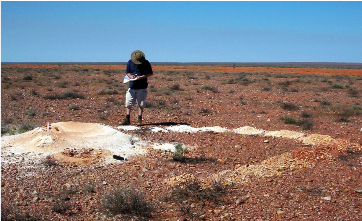
Plate 3. Logging of drill cuttings from completed auger hole. (Photo No. 407216)
