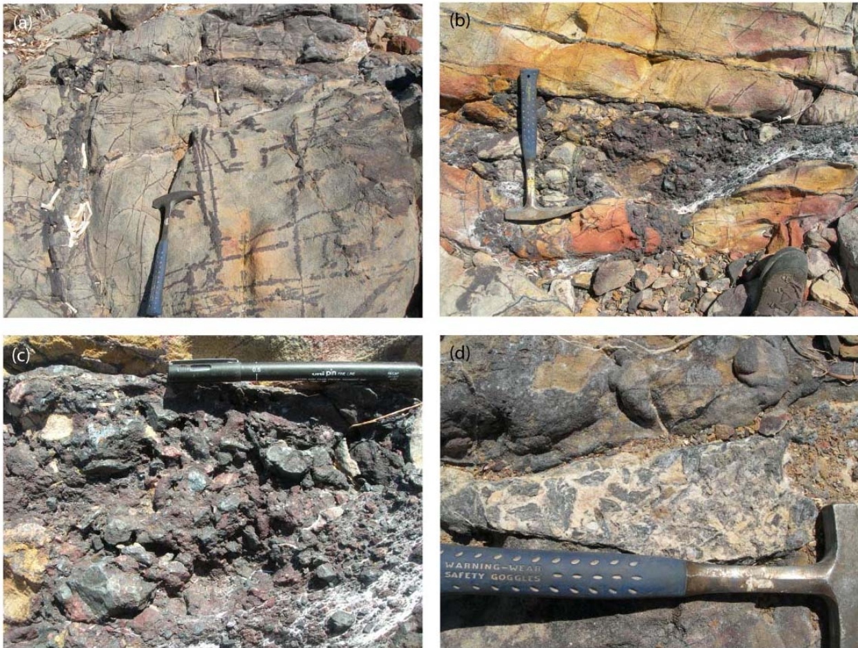
Figure 14. Haematite alteration in the Moonabie Formation. (a) N – S, E – W and subhorizontal haematite veining, looking N. (b) N – S striking breccia with haematite rich matrix, looking E. (c) Haematite breccia, looking E. (d) Vein with haematite fragments in a quartz matrix, looking E.
