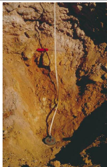
Plate 21: Pit GCP121, SE face, ~2.5-3 m (red marks at 2 m) with central logged and sampled profile marked by measuring tape (Lintern and Sheard, 1999b). (photo 45484).
