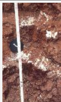
Plate 8: White alunitic seams in transported Cainozoic red-brown clay at Poona Mine (Hartley, 2000).
