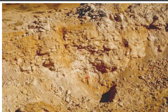
Plate 18: Pit GCP121, wide angle view, SE face with logged and sampled profile marked by measuring tape (Lintern and Sheard, 1999b). (photo 45481).
