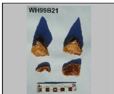
Plate 6: Dark rind lag clasts of silicified Cambrian sandstone from the unconformity contact with overlying Cainozoic clay, Wheal Hughes Mine, SW face (Hartley, 2000).
