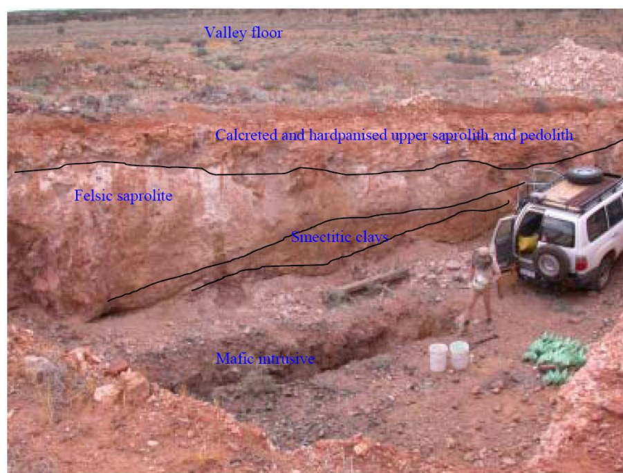
Figure 55: View of Benchmark 9 (Ian's Mine) S face in foreground with valley and dunes in background. Fifteen profiles were sampled from the S face and the data generated are contoured in Figure 56a-c. The vehicle is parked on pit's access ramp, facing west.
