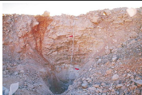
Plate 26: Pit GCP100, wide angle view, NW face with logged and sampled profile marked by measuring tape (Lintern and Sheard, 1999b). (photo 45504).
