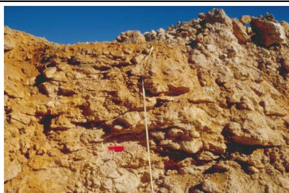
Plate 19: Pit GCP121, SE face, top metre (red mark at 1 m) with central logged and sampled profile marked by measuring tape (Lintern and Sheard, 1999b). (photo 45482).
