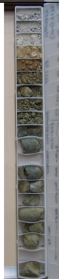
Figure 47: Benchmark 8 , aircore chiptray samples (exploration drillhole BG-32) with key regolith features indicated. Sample interval = 2 m.
