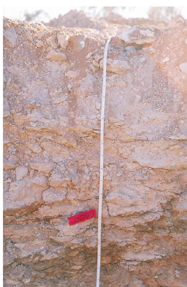
Plate 27: Pit GCP100, NW face, top metre (red mark at 1 m) central logged profile indicated by tape (Lintern and Sheard, 1999b). (photo 45505).
