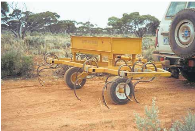
Ripper/scarifier set up and ready for use (in jacked-up position). (Photo 46538)
