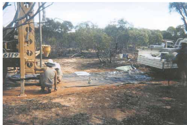
Pinkawillinnie drillsite; plastic liner minimises dispersion of dust and cuttings into the surrounding environment. (Photo 47067)
