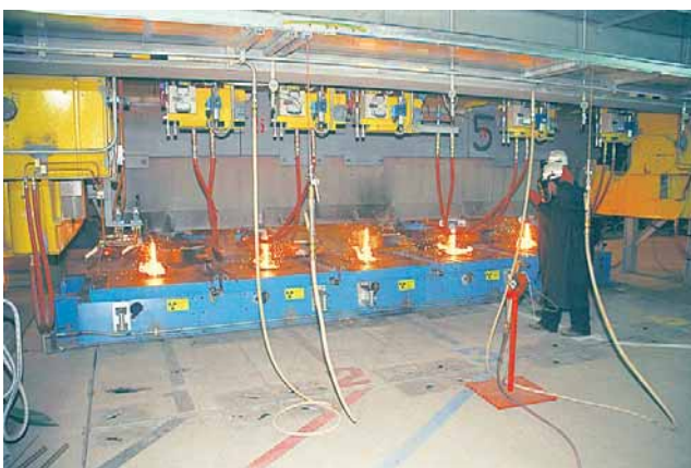
BHP employees watch as five strands of liquid steel are poured into Whyalla Steelworks' new $83 million billet caster. (Photo 46834)
