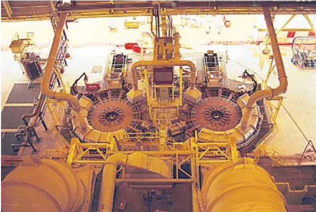
Dual wheel casting system in the new smelter building, Olympic Dam Mine. (Photo 46509)
