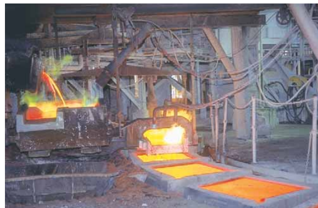
Casting copper anodes in the original Olympic Dam refinery. (Photo 44156)
