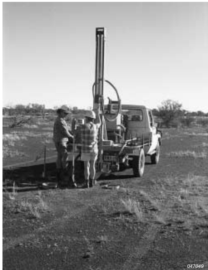
Auger sampling of calcrete at Hawks Nest.
