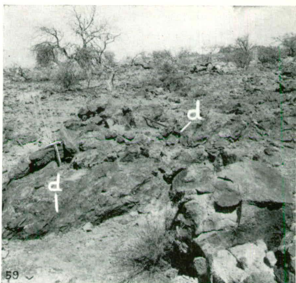
FIG. 59—SPRING HILL URANIUM PROSPECT General view of the main mineralized area—Out- crop rich in davidite (d) in left foreground
